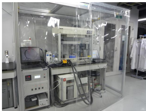
Fig.6 Chip bioreactor system for maturation of retina pigment epithelial cells
